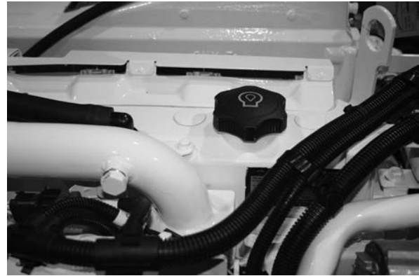
Left Side Oil Filler and Dipstick Location
